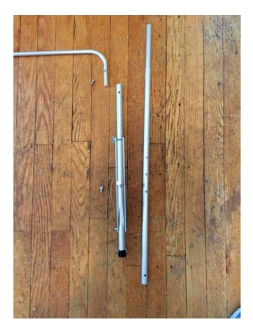
1. Begin by setting up the forward "U" shaped rod as shown above, with the right leg and riser positioned as above. The left leg and riser should be similarly positioned on the left.
