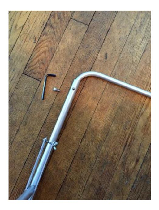
2. Now, starting on the left side, insert the left end of the forward rod into the front of the left leg (see picture above). Using the Allen wrench supplied and pictured above, insert the socket cap screw (shown above) into the hole and tighten.
